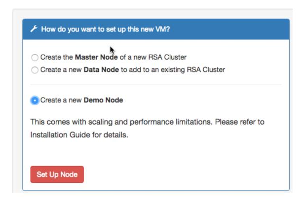
3. From Ruckus Smart Analytics, select the Create the Master Node of a new RSA cluster, Create a Data Node to add to an existing RSA Cluster or Create a new Demo Node as appropriate.
