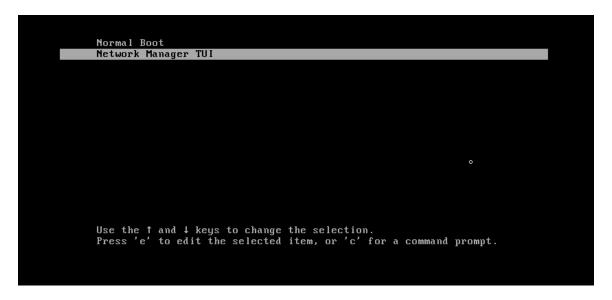
Select Network Manager TUI to the set the static IP address, and Normal Boot to start SCI.
