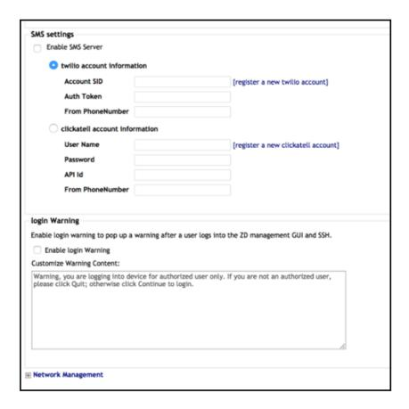
The path to get to this screen in the ZoneDirector Web UI is **Configure > System**. The **Enable login Warning** box is located in the bottom half of the screen.
