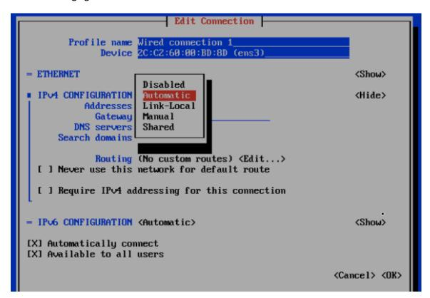
8. Change the connection type for the IPv4 Address to **Manual**.
